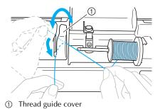
Pass the thread under the thread guide plate, and then pull it up.
